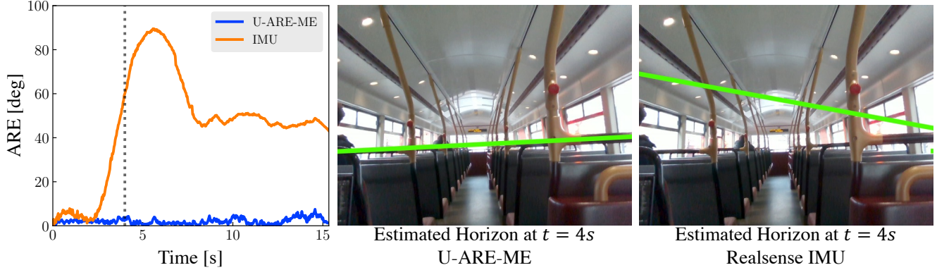
Figure 6. IMU sensors are prone to drift especially in non-inertial frames of reference (e.g. inside a moving vehicle). The horizon line in each image represents the up-vector inferred from our proposed method (middle) and an IMU sensor (right).
