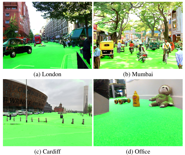
Figure 7. Even in non-Manhattan scenes, our framework can optimise the rotation such that the global up direction is aligned with the surface normal of the ground plane. It can thus be used to accurately segment the ground plane, shown here in green, which can be useful for many applications in robotics.
